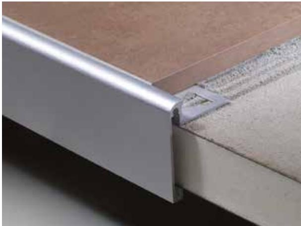
PLANOTEC BP extruded silver anodized profiles present a technical contour for tiled kitchen countertops. The molded profile section trims and protects the tile edge while covering the entire thickness of the countertop. This profile fulfills both technical and aesthetic expectations. External aluminum corner joints available.
